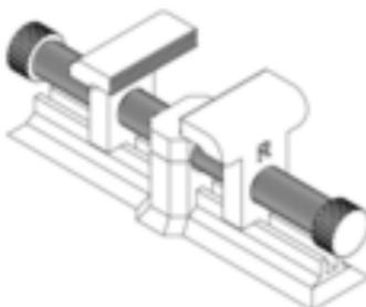
Thread on both clamps and Thread each clamp all the way down the thread going in a back and forth motion on any areas that give resistance to make sure it threads smoothly once fully assembled. Try to make sure they are both the same distance from the middle to ensure your clamped workpiece is always centered.
